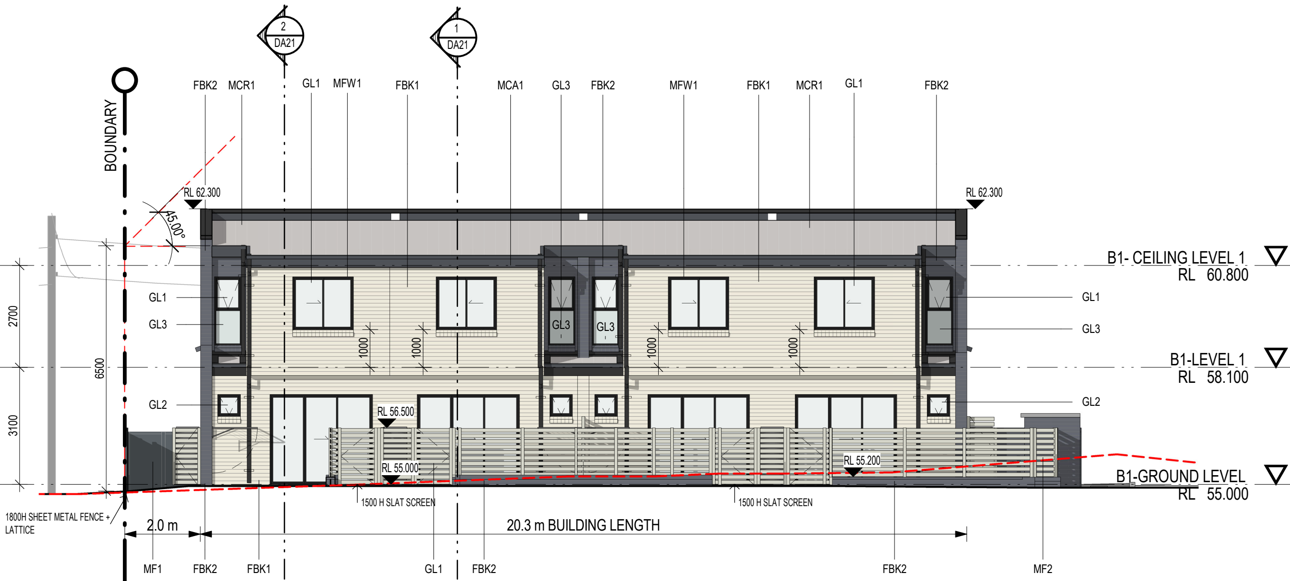
ELEVATION - INTERNAL WEST UNITS 1 TO 4 1 : 100
